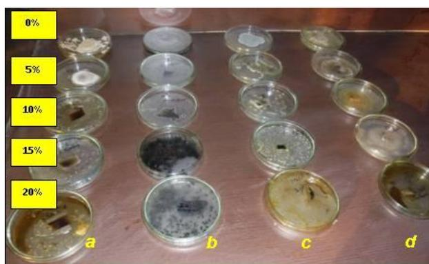
**Fig 3:** Growth determination of the fungi hydrocarbon growth capability in different concentration of kerosene
